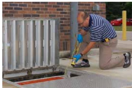
Figure 4: Suspending an OdaLog® H<sub>2</sub>S Monitor in the Headspace of the Wet Well
